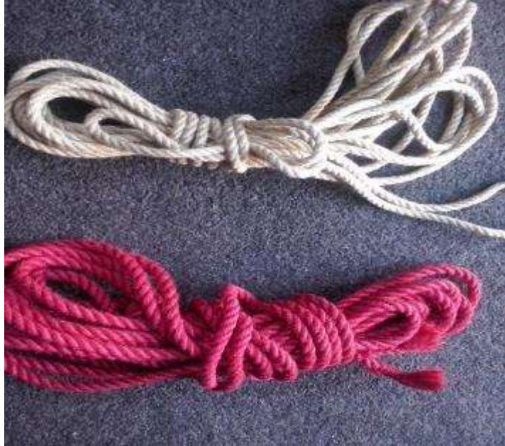
Above; undyed five mil tossa jute; below, 6 mil dyed tossa jute
